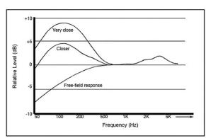
Proximity effect is a characteristic of all directional microphones; it is a rise in low-frequency response that increases at closer working distances. While this can be used to good effect, particularly with male voices to give them
