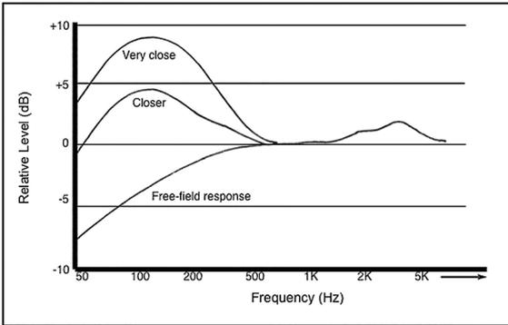
Proximity effect is a characteristic of all directional microphones; it is a rise in low-frequency response that increases at closer working distances. While this can be used to good effect, particularly with male voices to give them
