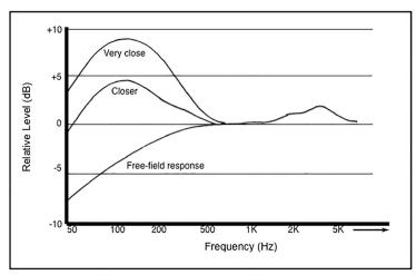
Proximity effect is a characteristic of all directional microphones; it is a rise in low-frequency response that increases at closer working distances. While this can be used to good effect, particularly with male voices to give them an enhanced richness and depth, the potential trade-off is reduced articulation or clarity that can result from the masking effect on the treble due to "excessive" bass boost.
