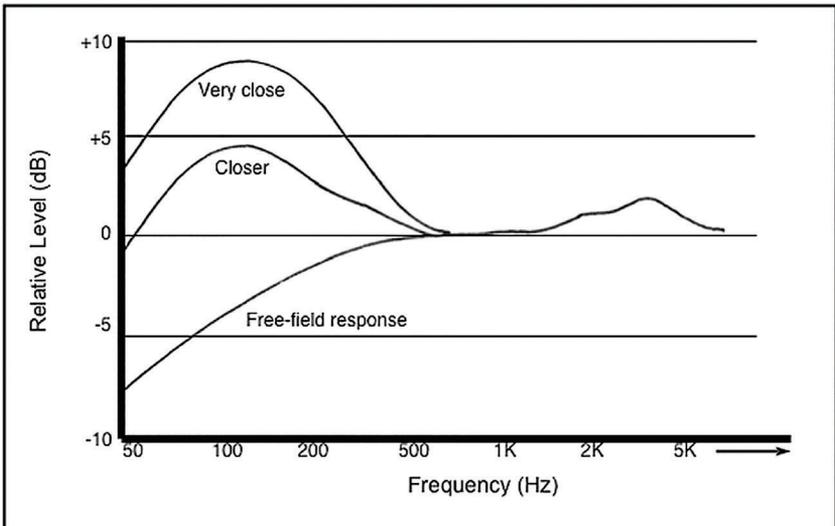
Proximity effect is a characteristic of all directional microphones; it is a rise in low-frequency response that increases at closer working distances. While this can be used to good effect, particularly with male voices to give them an enhanced richness and depth, the potential trade-off is reduced articulation or clarity that can result from the masking effect on the treble due to “excessive” bass boost.
