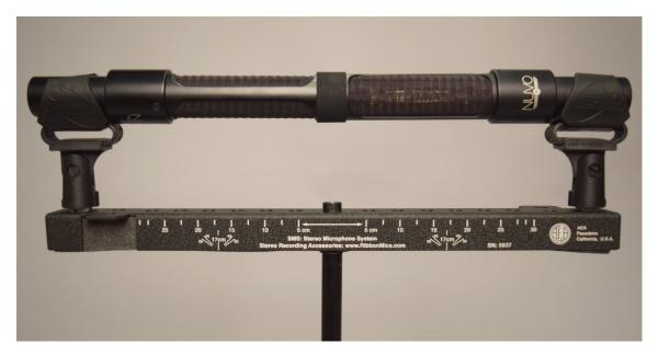
4) Now, attach the array to your mic stand, using the 5/8-27 female to 3/8-16 (EU) stand adaptor. If needed, use the Posi-Lok adjustable angle adaptor to allow adjusting the angle of the entire array.
